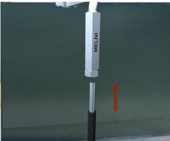
3. Tighten nut to specified torque.
